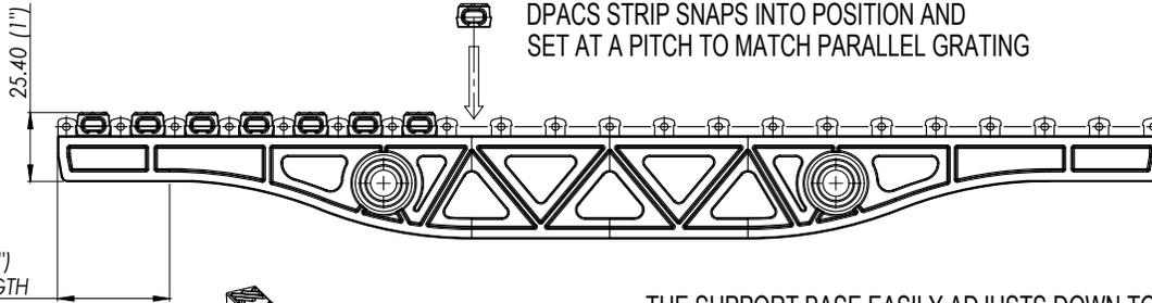
DPACS STRIP SNAPS INTO POSITION AND SET AT A PITCH TO MATCH PARALLEL GRATING
