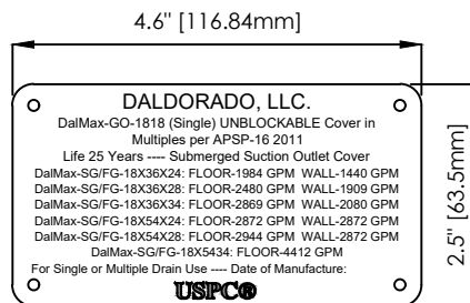
SPECIFICATION PLATE DETAIL
