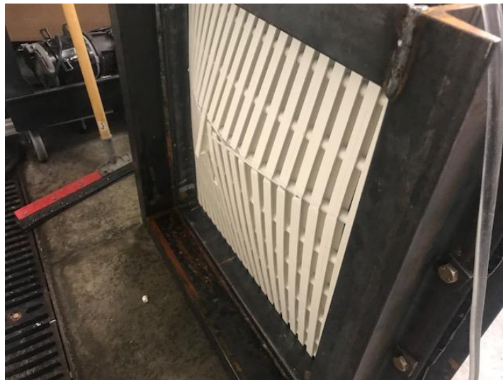
Pressure Differential and Point Impact Test Result for Suction fittings model no. DMD-FG-2424 (24" by 24" frame)
